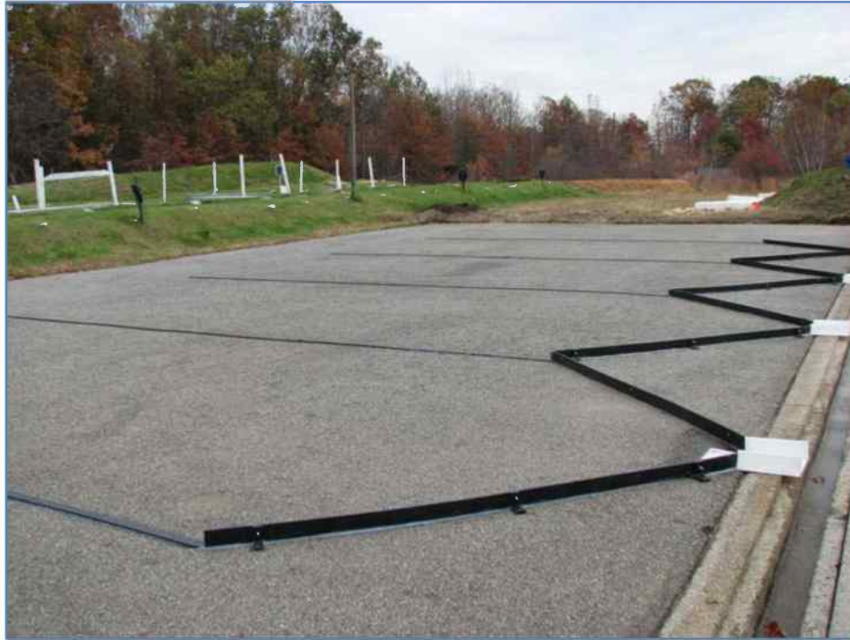
Figure 10. The four test plots at EPA's Urban Watershed Research Facility prior to sealing.
