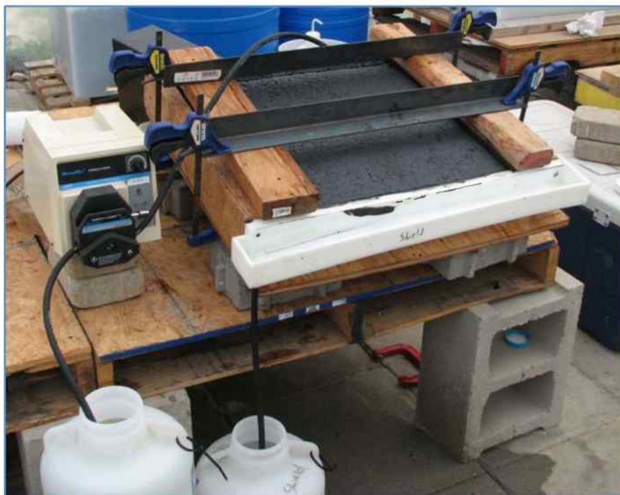
Figure 3. Sealed asphalt panel with rainwater delivery apparatus, angled to promote runoff.
