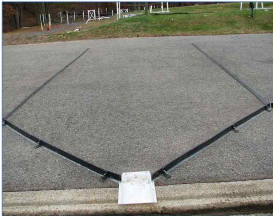
Figure 9. Asphalt test plot showing the flow directors and the ramp into the drain.
